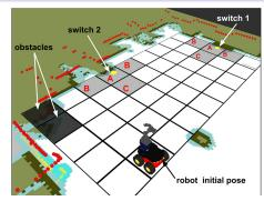
Domestic robot ensures light switches are off Abstractization to high-level control (physical actions implemented by low-level controllers)
